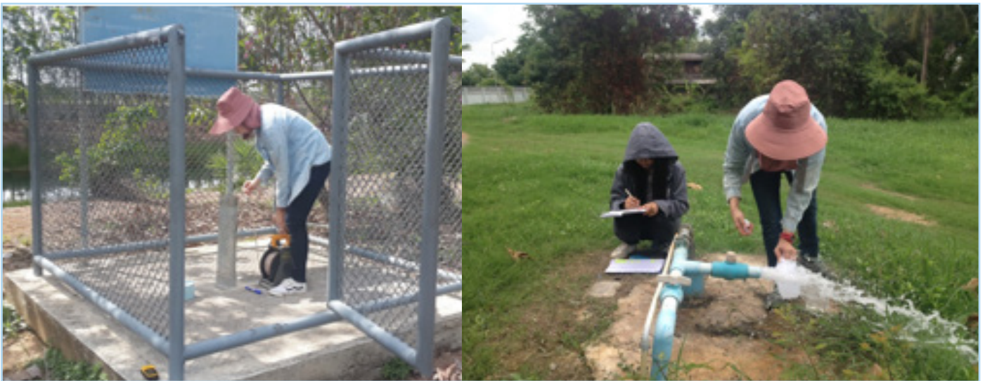
Figure 34 – Protection of the observation well (left) and the process of reading the measurements (right)
