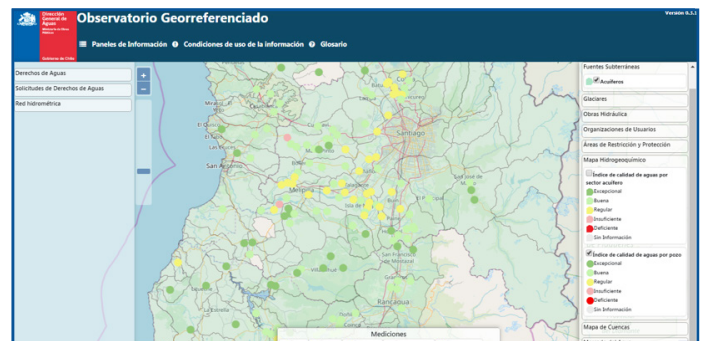
Fig. 25 – Web platform of the Hydrometric Network, coloured dots show the quality of the monitoring wells
