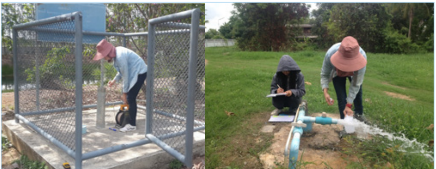
Fig. 186 – Protection of the observation well (left) and the process of reading the measurements (right)
