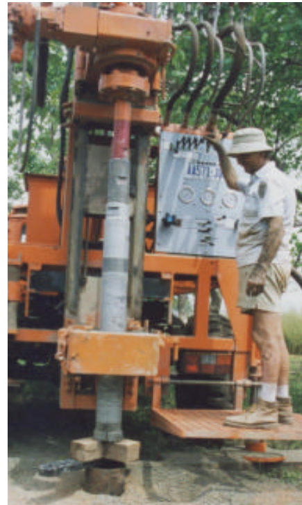
Down the hole hammer with button bit attached
