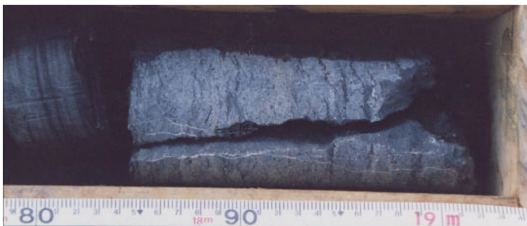
Figure 5.8 A cored sample showing an open fracture in limestone, associated with calcite veining.
