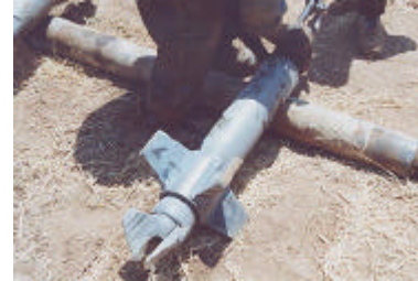
Drag bit with reamer for drilling unconsolidated formations
