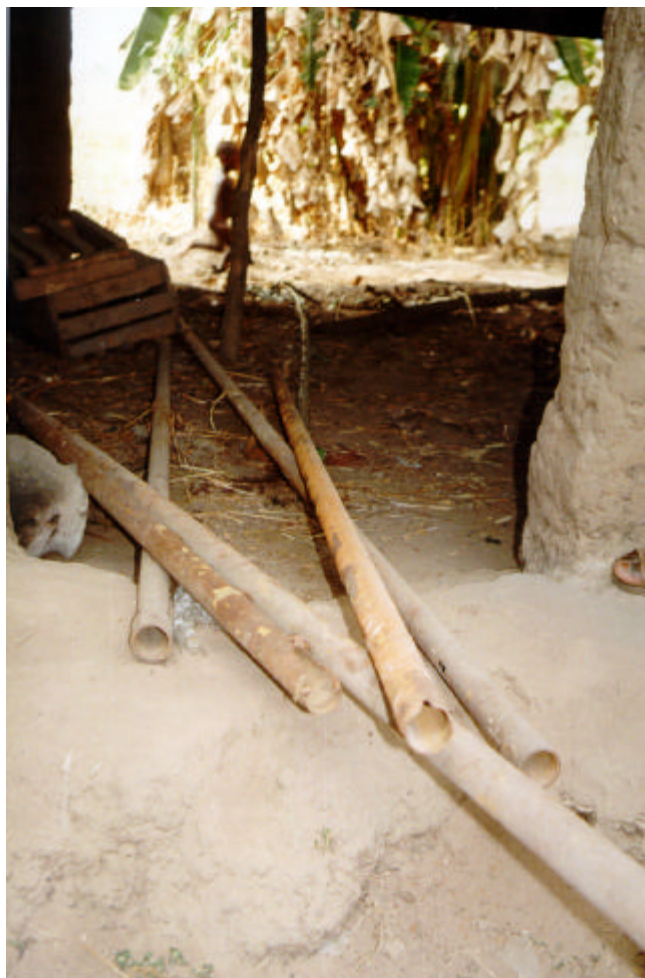
Figure 7.2 Highly corroded rising main from a borehole with TDS greater than 3000 mg/l. New rising main corroded within one year.
