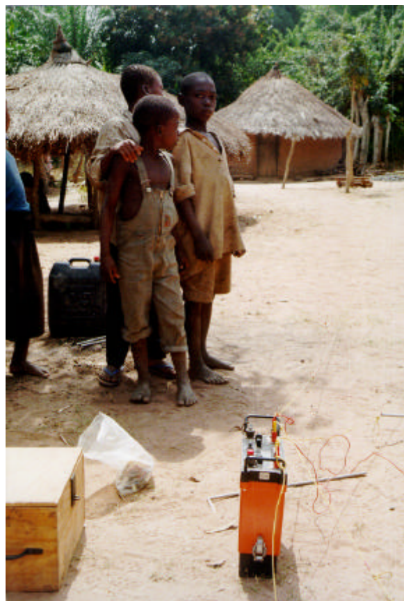
Figure 4.20 The instrument stays at the midpoint and cables run out to either side.
