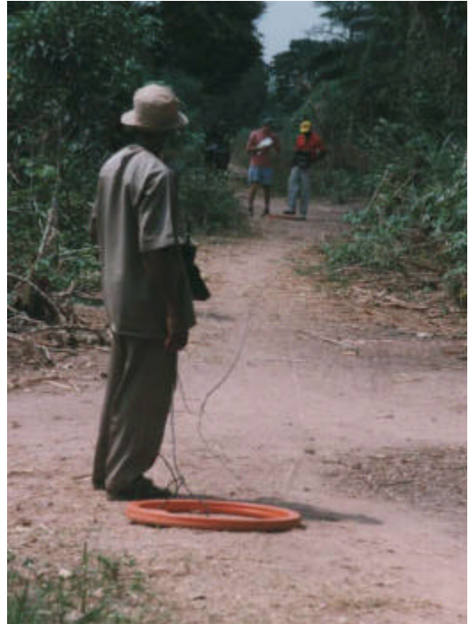
Figure 4.9 The EM34 being used with the coils horizontal.
