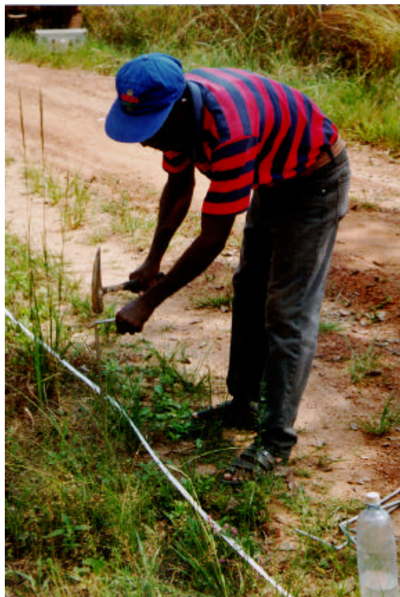
Figure 4.19 Electrodes have to be hammered in and sometimes watered to ensure good electrical contact with the ground.
